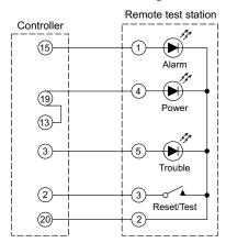
Remote test station wiring
